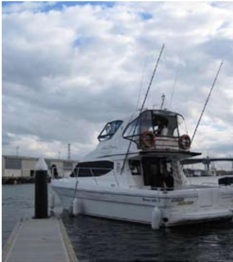
**5** Once you're abeam of your berth, place the starboard engine in reverse and the port engine in neutral. This will slow down your forward movement and direct the stern to port, while your bow will start to swing to starboard. Your boat should slowly move astern in a gentle arc to port, ideally angling your stern into the pen.
