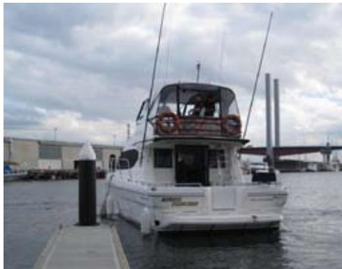
**6** Continue to move astern in an arc as you start to enter the pen. If you need to increase your turn rate, engage the port engine forward briefly while leaving the starboard engine in reverse. This should slow your vessel from going astern and cause the boat to pivot clockwise.
