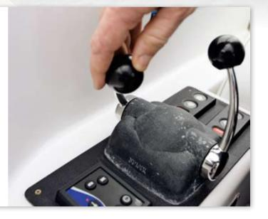
Coming in to tie-up on the starboard side and still heading in a straight line towards the dock at idling speed. Approximately a half-boat length away from the dock, place the port engine in neutral. We already have forward momentum, but with the starboard engine still engaged and the port engine now in neutral the boat swings in a gentle arc to port.
