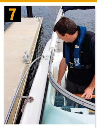
Once you are close to the dock, you can make some gentle corrections if necessary. For example, if it looks like you will go past the cleat, you can momentarily engage the port engine in reverse. Or if you lose forward momentum before the cleats are aligned you can momentarily engage the starboard engine forward. Either of these actions will have the effect of moving our stern nearer the dock.
