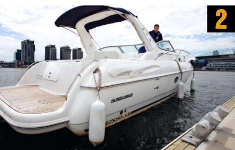
Once you've made your observations ensure your lines are ready and attached to the cleats on the boat. Always have your own lines ready and never rely on there being lines on the dock. Make sure fenders are attached and appropriately placed.
