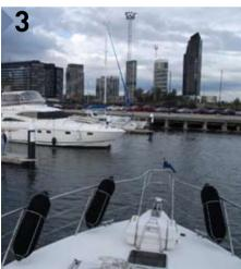
Approach the berth down the fairway at idle speed. When the vessel is travelling in a straight line, you'll know the rudder is centred. Now let go of the wheel and use only the engines to steer. Disengage the port engine, leaving the starboard engine engaged, to cause the vessel to swing gently to port. To go to starboard, disengage the starboard and engage the port gear.
