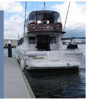
•10 Once you've reached the back of the pen, take a pre-prepared line, cast it over the cleat on the dock and tie off back to your boat. On a flybridge vessel, it's simpler if there's someone on board assist with this, but even singlehanded, it can be done without rushing around.
