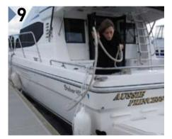
Once you've reached the back of the pen, take a pre-prepared line, cast it over the cleat on the dock and tie off back to your boat. On a flybridge vessel, it's simpler if there's someone on board assist with this, but even singlehanded, it can be done without rushing around.
